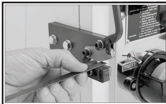
Figure 24. Using the blade shear to cut the blade.
